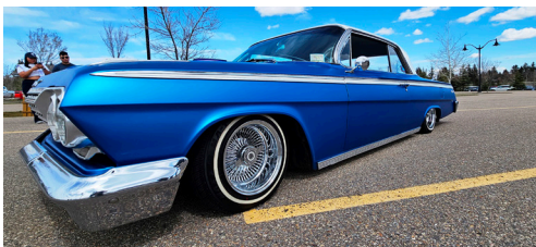
Vinyl-wrapped '64 Impala low rider with air suspension front and rear.
